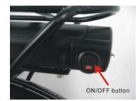
the on/off button on the battery to on. To turn off the bikes electrical system, switch the on/off button to off. (Please refer to the adjacent picture)
