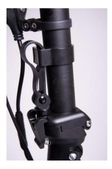
Then release the quick release clamp, located on the cross bar, and swing the clamp through 90 degrees around a vertical axis. Then push vertically down on the plunger assembly to uncouple the two halves of the folding locking mechanism and fold the two halves of the bike together.
